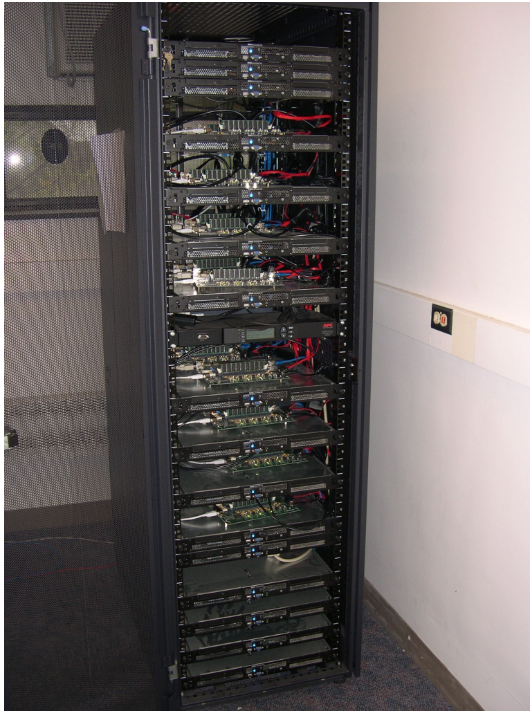
Figure 5.4 Griffin Cluster containing 16 Dell computers connected to 16 Digilent FPGA boards
